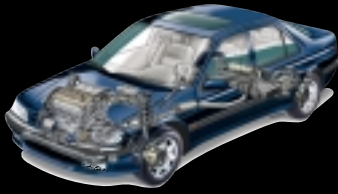
Hardening and tempering of engine and trans- mission parts. Curing of paint and brake-disc coatings. Bonding of body parts. Tube welding of exhaust pipes. Brazing of components. Magnet bonding in electric motors.
