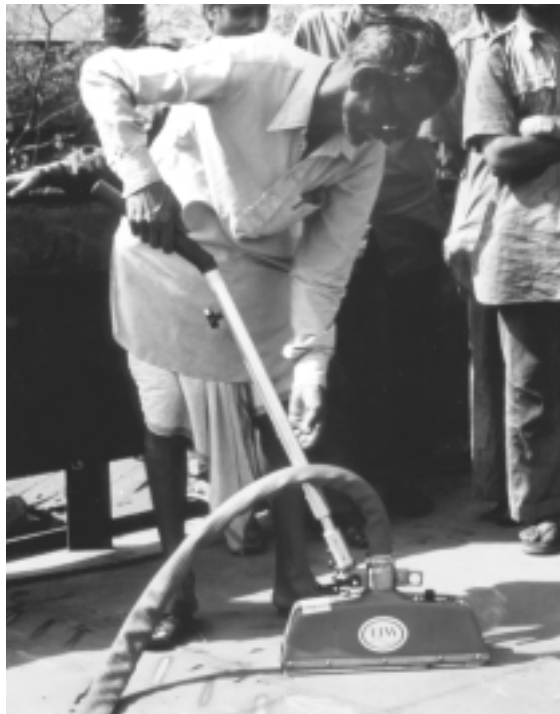
EFD Induction equipment has been used and trusted around the world for decades. This 1986 snap shows employees of Garden Reach Shipbuilders and Engineers Ltd. in Calcutta, India, testing their new ELVA TERAC 16 induction heating machine. The system was used for straightening ship hulls.
