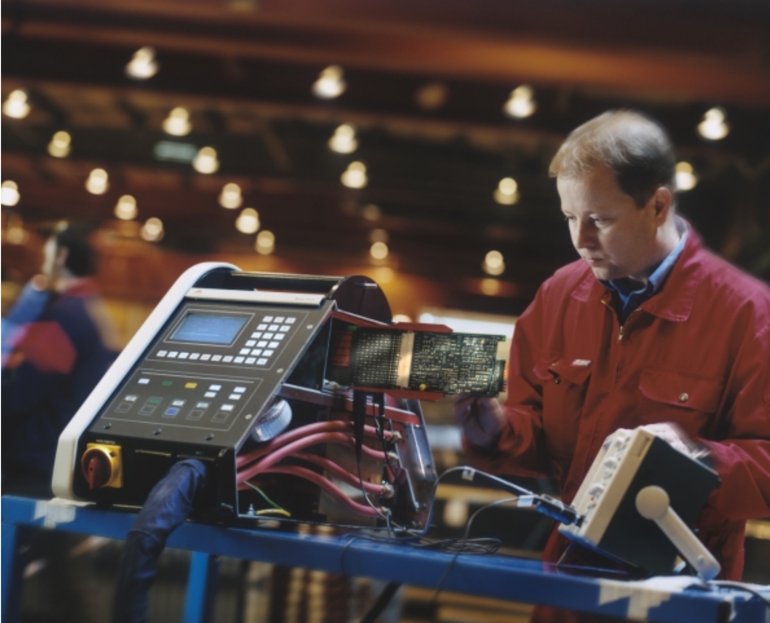
EFD Induction services range from pre-production planning and materials analysis to full preventive and corrective maintenance contracts. Here, one of our engineers upgrades an EFD Induction Minac mobile induction heating system.
